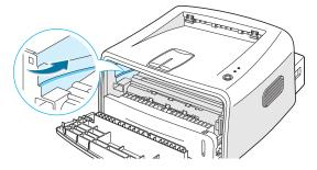
**5** Close the front cover. Make sure that the cover is securely closed. If it is not firmly closed, printing errors may occur when you print.
